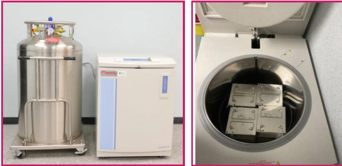
Fig-2 Cryovials With Different Samples Kept Inside Thermo Scientific CryoPlus Storage Systems (In Vapour Phase At -150°C To -170°C)
