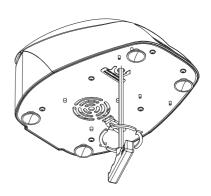
Disconnect the centrifuge from the main supply. Wait until the rotor comes to a standstill (this may take some time). Once the rotor has stopped, use the T-allene key from bottom side of the unit, rotate the T-allen key in counterclockwise direction as indicated in above figure this will open the centrifuge lid in case of emergency lid opening.
