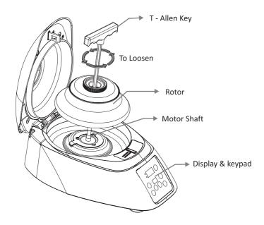
The rotor of the centrifuge is pre-installed. In case of any spillage, remove the rotor as shown in the above figure to clean the rotor and its chamber thoroughly.
