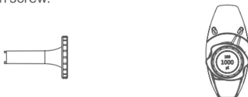
3. Remove volume adjustment knob by pulling it upwards.
