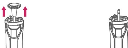
4. Place the calibration tool into the calibration grooves.
