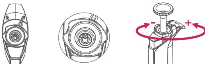
5. Rotate the calibration tool counter clockwise to increase and clockwise to decrease the volume.
