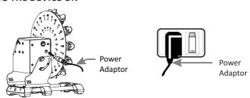
After connecting the power adaptor to back side of the device, switch the main power supply to "ON" & then switch the device on from the rear. Make sure that tubes are loaded properly before use.
