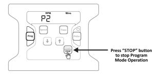
To leave Program mode, hold down the "Program" button again to turn OFF the Program mode. It will display "Prog off" indicating program mode is off.
