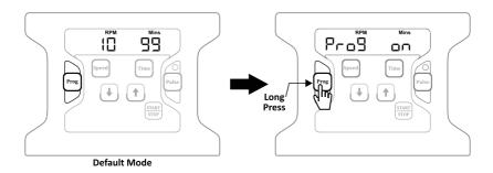
After a few seconds, the display will show "P1" and "speed & time value" alternatively. This shows that the current program is P1 with some RPM and time value.
