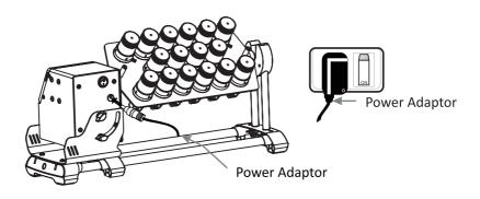
After connecting the power adaptor to back side of the device, switch the main power supply to "ON" & then switch the device on from the rear. Make sure that tubes are loaded properly before use.
