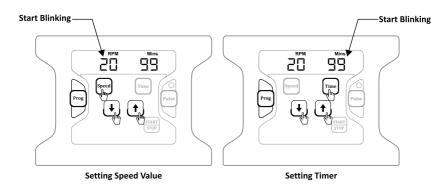
Speed and time value for that particular program is now saved. Press the "Start Button" to start the program mode operation. Once set RPM is reached, the program "Px" (with x = 1 to 9) and its "Speed" & "Time" value will display alternatively.
