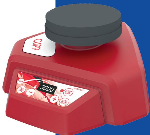
The CAPP Rondo Vortex Mixer is an indispensable piece of high-performance equipment designed to meet the rigorous demands of everyday mixing operations in any laboratory setting.
