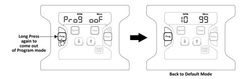
**NOTE:** On every restart, the device automatically comes out of program mode. It shows the last run default speed and time value.
